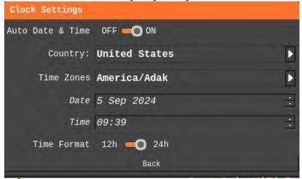
Note- Auto Date & Time is OFF by default. In order to enable Auto Date & Time the LiteNXT must be connected to the internet.
